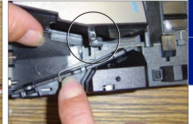
Move spring downwards to free the catch.
